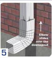
Attach the elbow OVER the downspout to prevent leaking.
