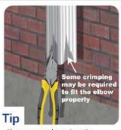
You many need to crimp the downspout with pliers to make it fit inside the elbow.
